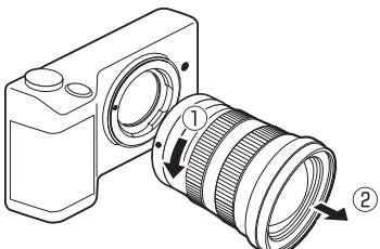
**Removing a lens from the mount-adapter**
